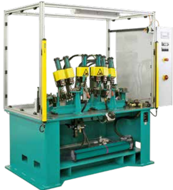
Press with TOX ® -Powerpackage X-KT-System: 1 pressure intensifier and 6 drive cylinders
